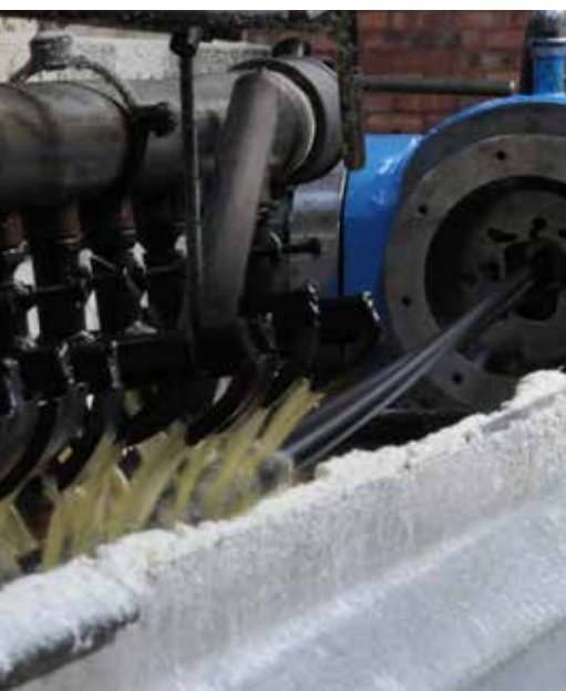
220° salt bath to accelerate the vulcanization process
