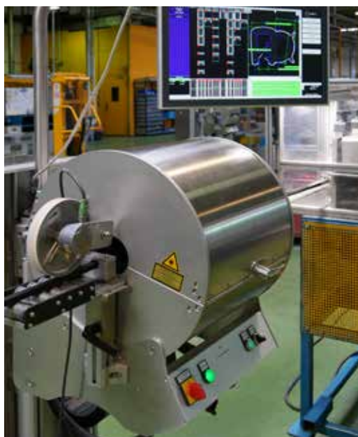
Permanent camera-based profile geometry monitoring (PIX-Argus)
