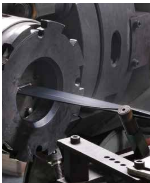
Extrusion die with emerging PVC profile
