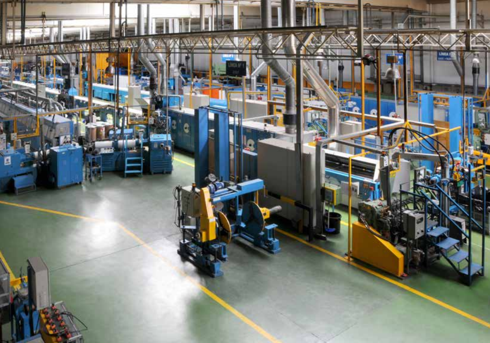
Rubber extrusion lines with salt bath and UHF vulcanization
