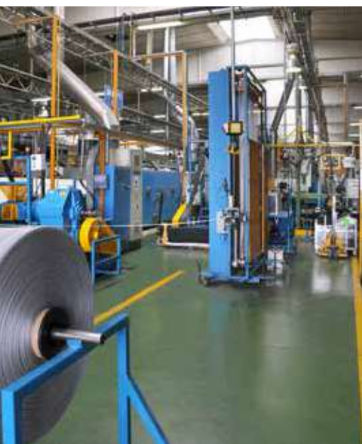
Wire spiral strip coil with intermediate storage
